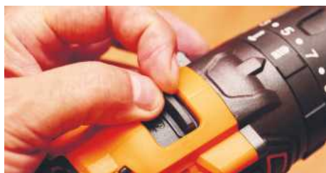
▲ Gear changing is set using a standard sliding switch
